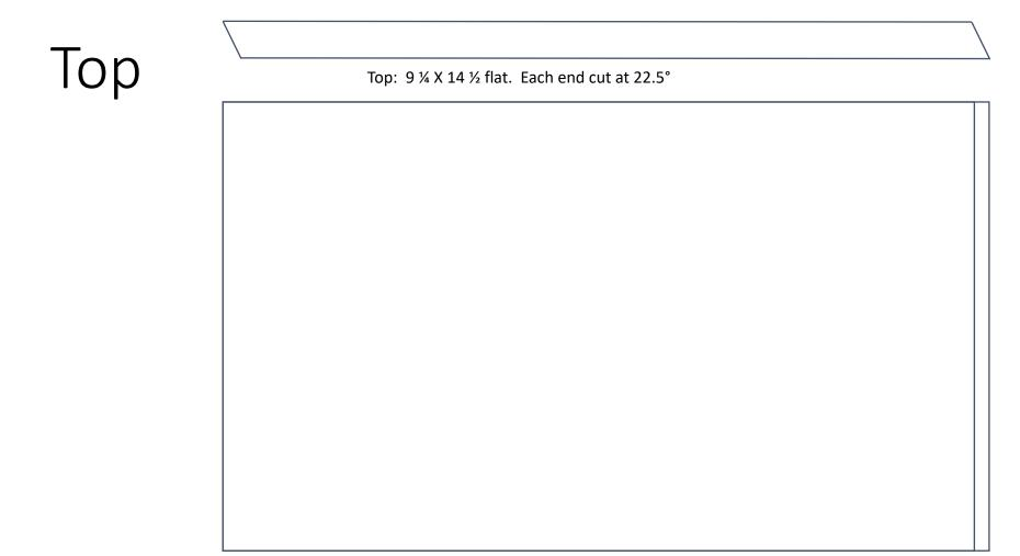
Out of an 8 foot 1X10 board, You can get 6 backs. The scrap from this can be used for hole guards.
